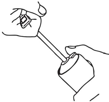
Pull on the push rod, actuate the safety catch, and push the push rod back into the cylinder.
