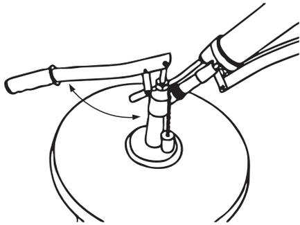
Fill the grease gun by activating the filling unit. Filling may cause the push rod to be pushed out of the grease gun cylinder.
