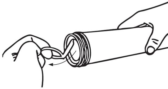
Only then tear off the cartridge's „pull-off“ closure and screw on the grease gun head.
