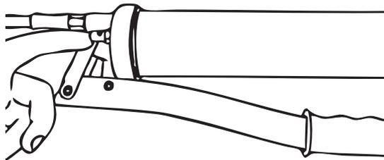
Remove air from the grease-containing section via the combined filling / air removal nipple on the grease gun head by loosening the gun head and cylinder (half a turn maximum) or by repeatedly actuating the hand lever.
