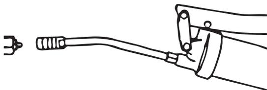
Position the grease gun with the hydraulic mouthpiece onto the grease nipple.
