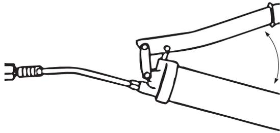
Actuate the hand lever to carry out the greasing process.
