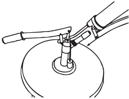
Place the grease gun onto the filling valve of the grease gun filling unit, and hold it in place with light counter pressure.
