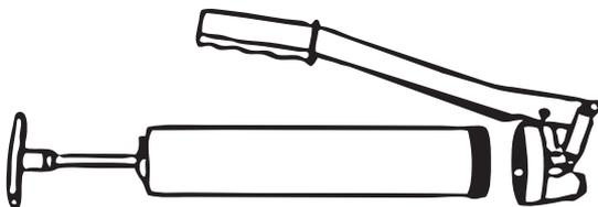
Pull back the push rod and unscrew the grease gun head.
