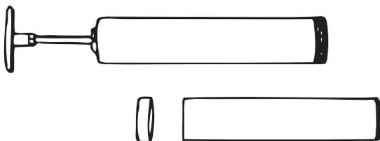
Remove the sealing cap from the full cartridge, and guide this into the grease gun cylinder.
