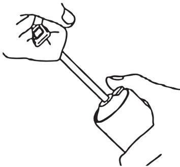
While pulling on the push rod, activate the safety catch and push the push rod back into the cylinder.
