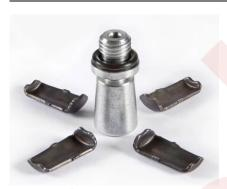
The steel jaws have one edge larger than the other, this is the edge that should go at the top (large end) of the cone. Placing a small amount of grease on the inner cone first can help to ensure that the jaws stick and don't fall out before being placed in the Grease Coupler.
