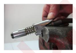
The vise, or pliers, will only have a small piece of the coupler to attach to, so don't be afraid to crank down on them and get a tight grip. When depressing the lever, you can see that the steel jaws of the seal kit are exposed and ready to be replaced.
