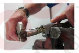
Using a pair of vise-grip pliers, get a very firm grip on the steel jaws of the seal kit. Because the jaws will be greasy and may rotate, you'll need to really squeeze them. Don't worry about damaging the jaws or the interior cone with your wrench, as these will all be replaced in a moment. Once you have loosened the interior cone by rotating the pliers counterclockwise, you can remove the pliers and continue to twist with your fingers.
