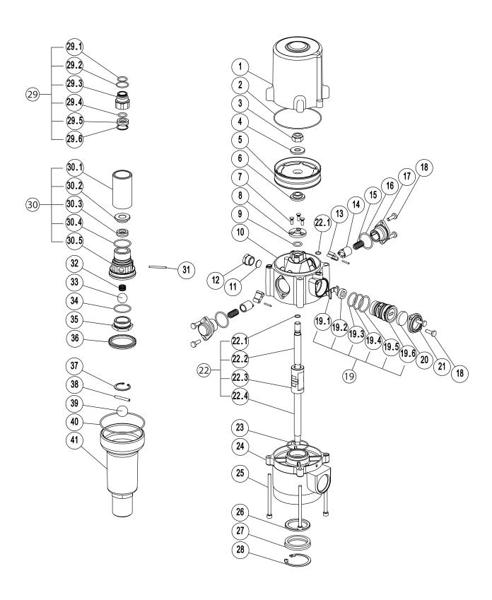
Fig. 11-1: Exploded View of the Pneumatic Oil Pump
