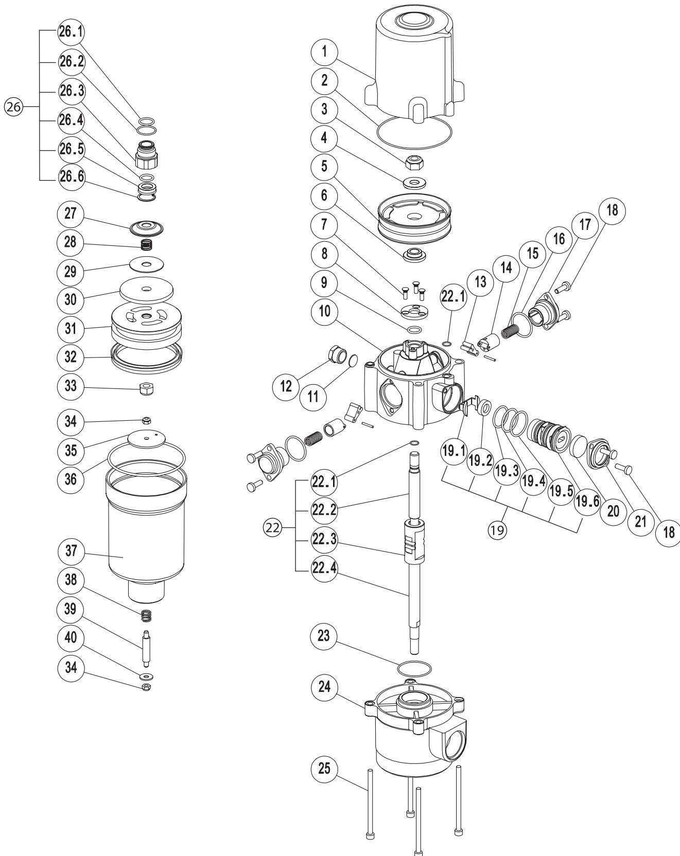
Fig. 11-1: Exploded view of the Pneumatic oil pump
